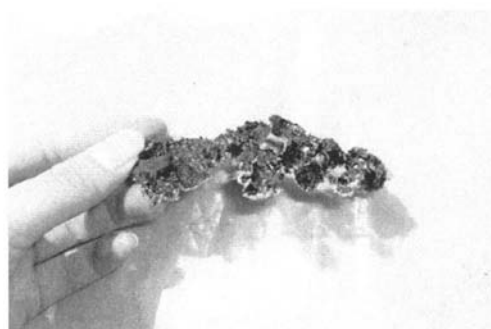
Fig. 7 Asphalt cutting back during curing.
