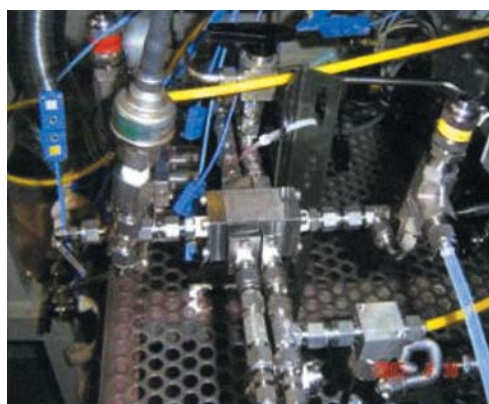
Fig. 20 Experimental apparatus of wax particle synthesis by crystallization method in the integrated double-zone micro heat-exchanger.
