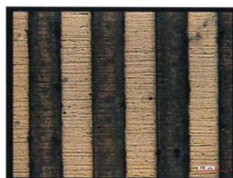
Fig. 3 Fluoroplastic micro particle coated micro channels observed by laser microscope.
