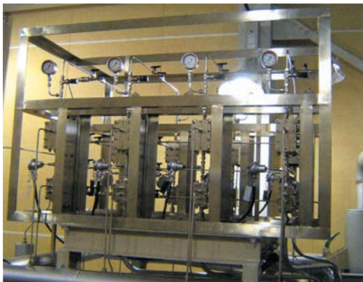
Fig. 19 The pilot plant of microreactor system for bi-phenol synthesis, which includes eight units of the micro mixer and the micro heat exchanger. Each series has 1 L/min processing capability.
